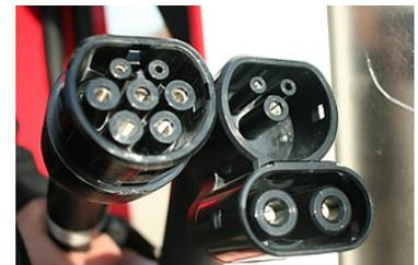
Europe/Worldwide Tesla Supercharger with dual cables: Type 2 for Model S/X and CCS Combo 2 for Model 3
