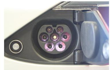
Type 2 compatible inlet implementing a three-phase AC charging and DC Supercharging on European Tesla Model S and Model X; a notch/teardrop-shaped keying planned for unprotected Mode 1 domestic charging was reused in 2019 for Supercharging
