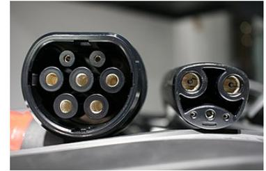
Tesla Supercharger outlets in Europe/Worldwide (left) and North America only (right).
